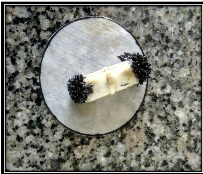
Fig. 2. Magnetic nature particles of the electro-coagulated sludge which is attracted to the magnetic bar during the batch experiment.
