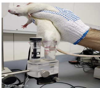
Figure 10. Photograph of the plethysmometer used for carrageenan-induced edema of hind paw in rats.
