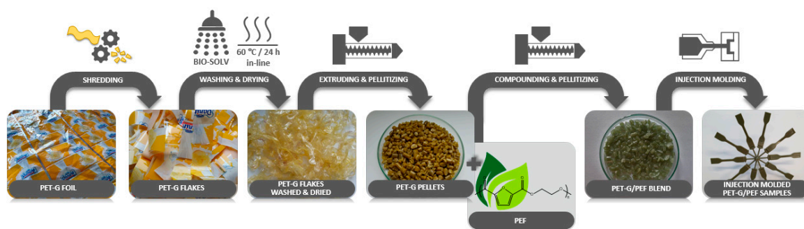
Figure 1. Schematic illustration of the preparation procedure of PET-G/PEF blends.
