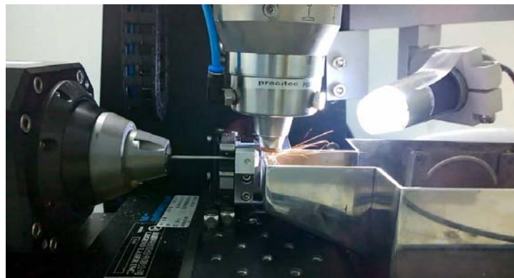
Figure 5. Cutting the design pattern of the rhombic-shaped channel stent onto a hypotube by laser.
