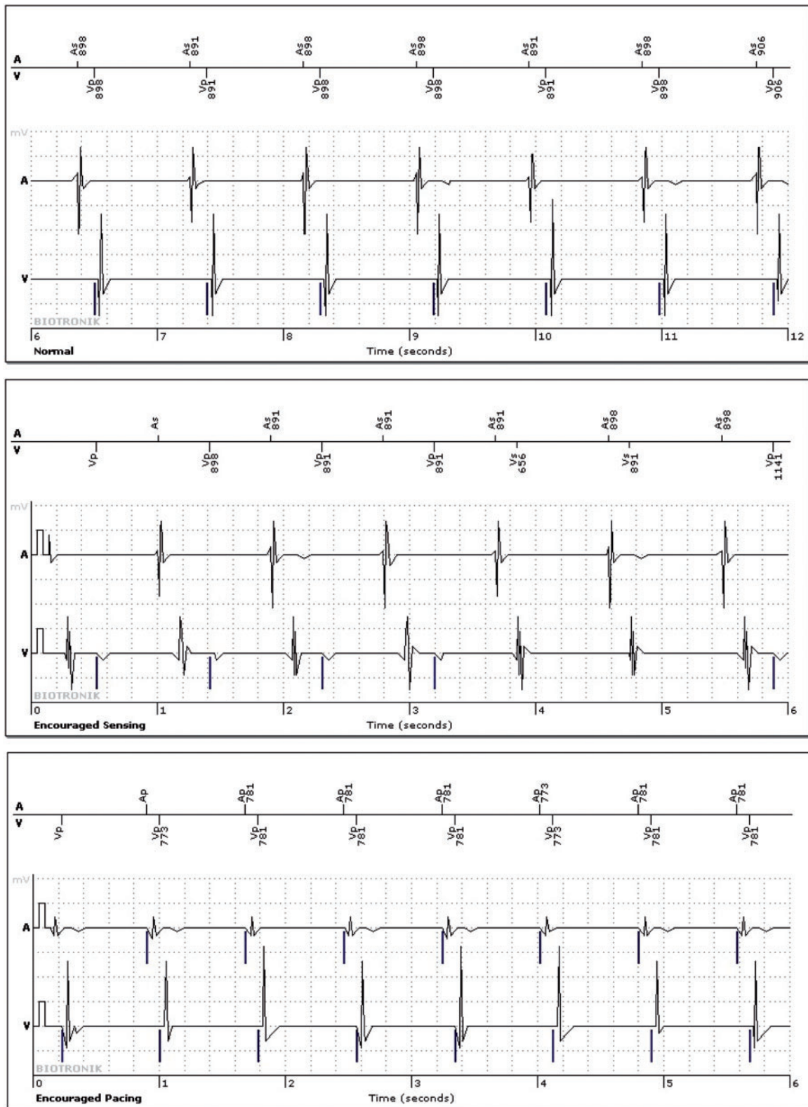
Figure 1 Added value of an active intracardiac electrogram (aEGM): The passive section ( normal ) of this periodic aEGM only displays effective atrial sensing and ventricular capture, which does not allow atrial capture and ventricular sensing assessment. Section 2 ( encouraged sensing ) reveals an undiagnosed intermittent loss of ventricular sensing on the first four and on the last ventricular beat, followed by a useless ventricular pacing, whereas Section 3 ( encouraged pacing ) allows to check effective atrial capture. Atrial and ventricular sensing and pacing functions are thus fully analysable thanks to all aEGM sections. The loss of ventricular sensing triggered an additional follow-up to adapt the ventricular sensitivity. Top line in each section: markers (Ap, atrial pacing; As, atrial sensing; Vp, ventricular pacing; Vs, ventricular sensing); A line, atrial electrogram; V line, ventricular electrogram. N.B.: For editorial reasons, only the first 5 s (instead of 10 s) of each aEGM section are displayed.
