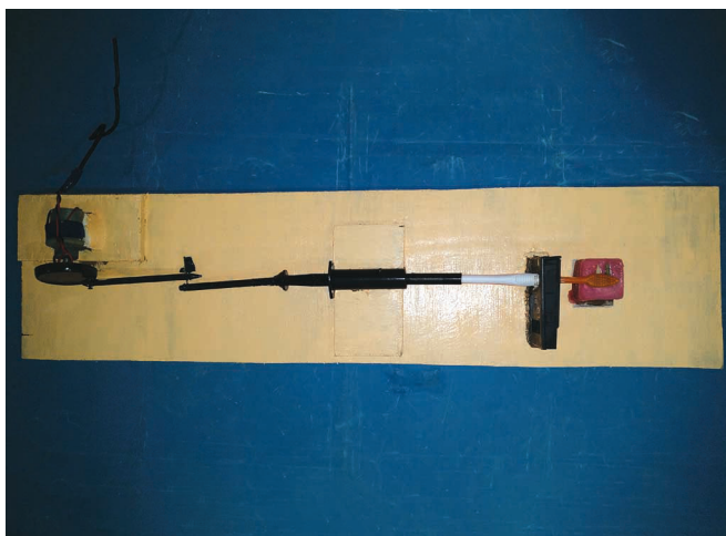
Fig. 2: Customized automated toothbrushing model
