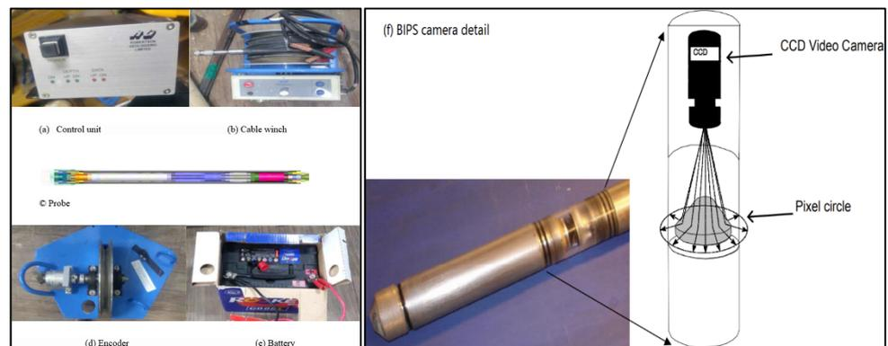
Figure 22. Main equipment accessories of BIPS system, (a) control unit, (b) cable winch, (c) probe, (d) depth encoder, (e) battery, (f) BIPS camera detail.
