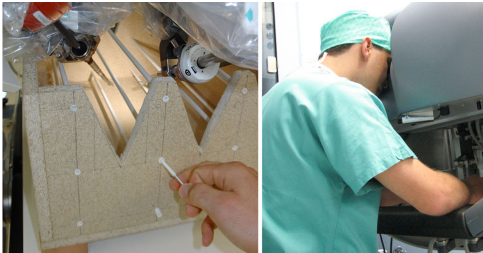
Fig. 4 Left Static da Vinci—magnetic sensors were pulled through a PVC tube. Right da Vinci ® was constantly in motion using the da Vinci console
