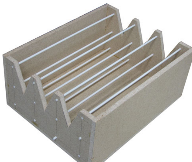
Fig. 1 Wooden metal-free measuring facility with 12 polyvinyl chloride (PVC) tubes, thus enabling laparoscopic instruments to be used between the tubes
