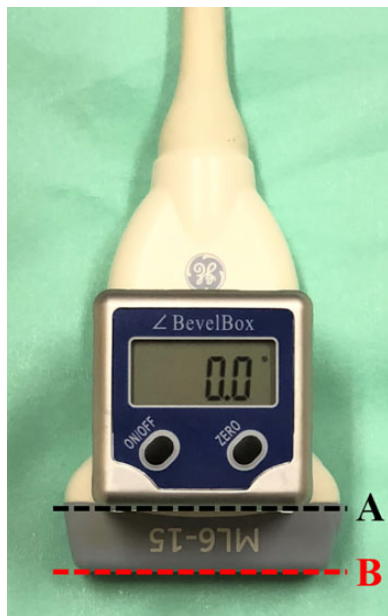
Figure 1. The ultrasound transducer with a digital inclinometer. A digital inclinometer was fixed onto the anterior surface of the transducer to verify that the inferior surface of the inclinometer (line A) is parallel to the transducer lens (line B).
