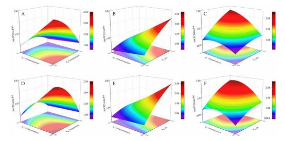
**Figure 2.** Response surface models for the response estimated based on two experimental factors keeping the third factor at its central level. Charts for Genapol X-080 (A–C) and Tergitol 15-S-7 (D–F).
