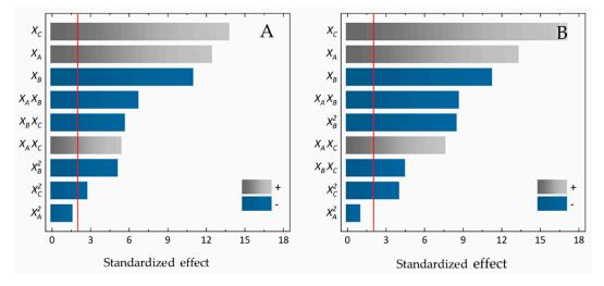
**Figure 1.** Analysis of the effects of the Box-Behnken factorial design. Pareto charts with standardized effects of three experimental factors, in decreasing order of importance (in absolute value) for the phenylethyl isothiocyanate (PEITC) content response. Genapol X-080 (**A**) and Tergitol 15-S-7 (**B**) aqueous micellar systems (AMSs). The vertical red lines represent the threshold of significance (p = 0.05) for 32 degrees of freedom.
