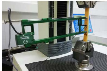
Figure 3. The tensile test assemblage of a sample from the hybrid resin.
