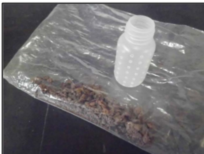
Figure A1. Put pulp in polyethylene plastic bag and make pulp into small particles (diameter 5–10 mm).
