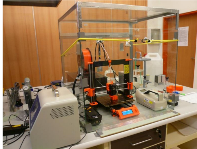
Figure 1. Glass box with printer and measuring instruments.
