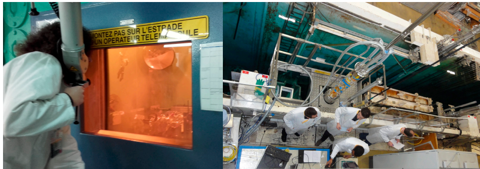
Figure 11. Picture of IRMA (left) and BRIGITTE (right) facilities used for irradiation of optical fibre sensors.
