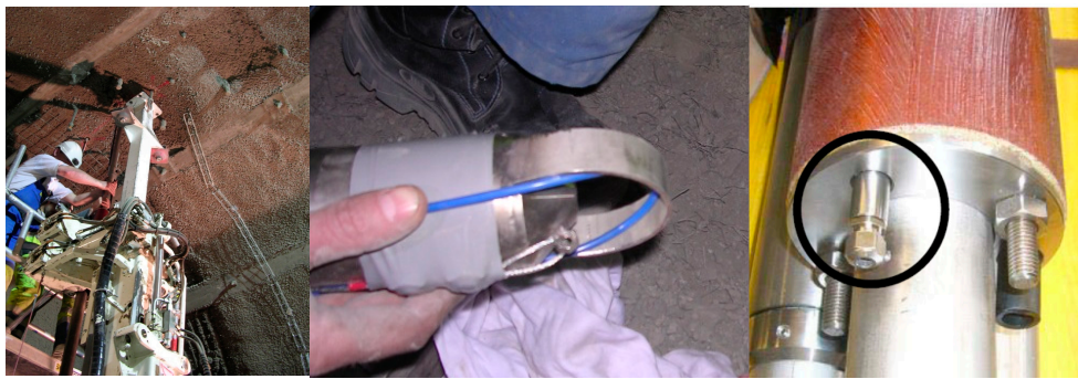
Figure 14. Pictures of distributed temperature system implementation inside vertical borehole ( left ). Example for a curvature guide ( middle ) and connector ( right ) to get the sensing cable through packers.
