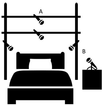
Figure 2 Microphone set-up at the top end of the bed. (A) Two microphones for high fidelity recordings (Earthworks M23) are placed at different heights at the midline of the bed. (B) Two microphones for average quality recordings (Behringer ECM8000) are placed at the same height at the sides of the bed and one on the night stand.
