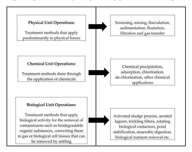
Figure 1. Summary of wastewater treatment unit operations. Source: [18,21].
