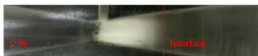
(a) Cavitation cloud distribution in a Venturi (Experiment photograph courtesy of Xiaolong Zhu et al. Copyright 2017) 18
