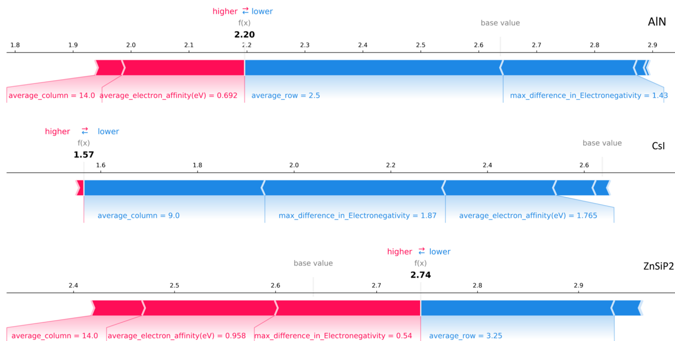
Figure 7. Visualization of the Shapley values of the SVR model of compounds AlN (top), CsI (middle), and ZnSiP 2 (bottom). Bars in red indicate that this descriptor “pushes” to increase the prediction; bars in blue indicate that this descriptor “pulls” to decrease the prediction. The base value represents the value that would be predicted when no feature is known for the current output, i.e., the mean prediction of the test set. Only descriptors with top contributions are annotated.
