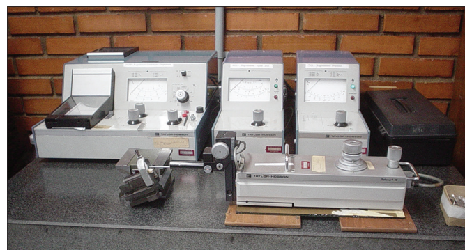
Figure 1: Roughness tester, Talysurf 10, Rank Taylor Hobson.
