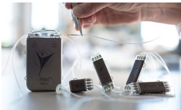
Fig. 2 Implantable components of the NNP system. The package on the left is the PM containing three Li-ion rechargeable cells. Smaller packages are remote modules. A network cable connects all components for communication and powering
