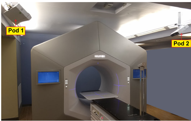
FIG. 2. Configuration of the SGRT pods on the Halcyon vault and the circle pattern used for daily and monthly calibration. SGRT, surface guided radiation therapy.
