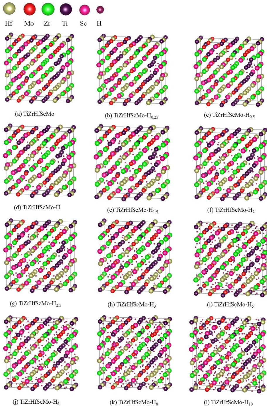
Figure 2. Illustration of schematic views of (a) the HEA TiZrHfScMo; (b–l) TiZrHrScMo-H x , where x is the number of hydrogen atoms per formula unit. The yellow, red, green, purple, and pink spheres represent Hf, Mo, Sc, Ti, and Zr atoms, respectively. The hydrogen atoms are represented by the smaller wine-colored spheres.
