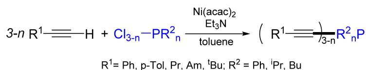
Figure 3. General scheme for a nickel-catalyzed cross-coupling reaction with terminal alkynes.
