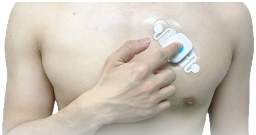
Figure 2. The electrode location for ECG monitoring using the CarePatch™ ECG patch.
