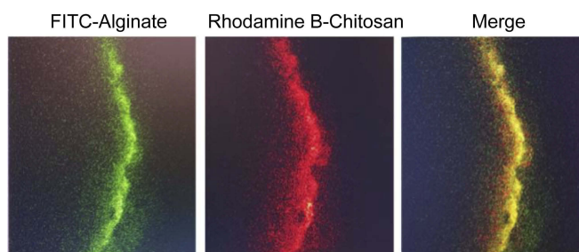
Figure S2 Laser scanning confocal microscopy images of a wall section of catechol-27–chitosan/barium sulfate microcapsules under different excitation wavelengths. Abbreviation: FITC, fluorescein isothiocyanate.
