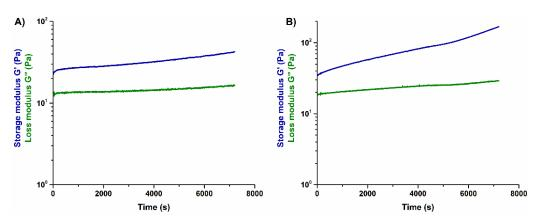
Figure 2. Visco-elastic properties of GEN-Coll solutions containing 0.1 wt.% (A) and 0.2 wt.% (B) of genipin, at 10 °C.
