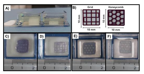
**Figure 9.** Images of 15 wt.% Alginic acid bath (**A**), scaffold design (**B**) and printed scaffolds after incubation at 37 °C for 24 h: GEN-Coll/MBG\_Sr4%, T1 and T2 (**C**,**D**, respectively) and GEN-Coll/nanoHA, T3 and T4 (**E**,**F**, respectively). Blue coloration of scaffolds is indicative of genipin crosslinking. Scaffold measurement  $10 \times 10 \times 1$  mm.
