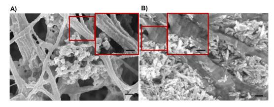
**Figure 10.** FE-SEM micrographs of produced scaffolds after freeze-drying. (A) GEN-Coll/MBG\_Sr4% and (B) GEN-Coll/nanoHA. Collagen D bands seen in both samples and zoomed in on area delimited by the red squares. Scale bar 100 nm.
