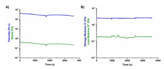
**Figure 8.** Variation of viscosity and visco-elastic properties of 15 wt.% alginic acid bath with time, at 23 °C, (**A**) viscosity and (**B**) viscoelastic modulus.
