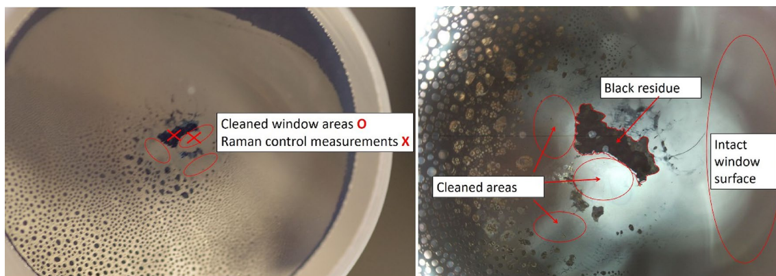
Figure 6. Rubidium cell window after laser cleaning; a small part of the black deposit is left for the purpose of control measurements. The Raman spectroscopy analysis was performed at the locations marked with X.
