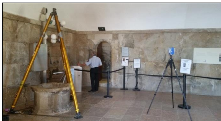
Figure 10. Structure required to access the cistern.
