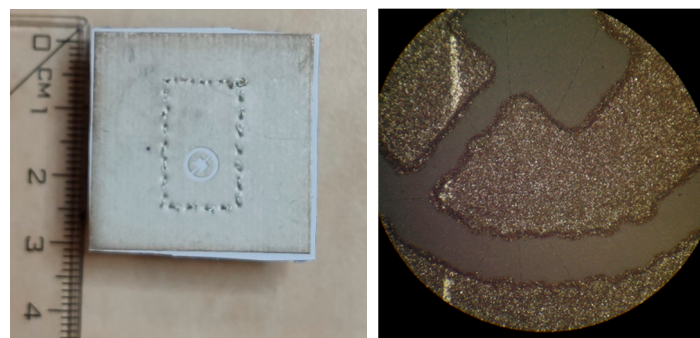
Figure 9. Photograph of the screen-printed antenna (left); microscopic view of the slot (right).
