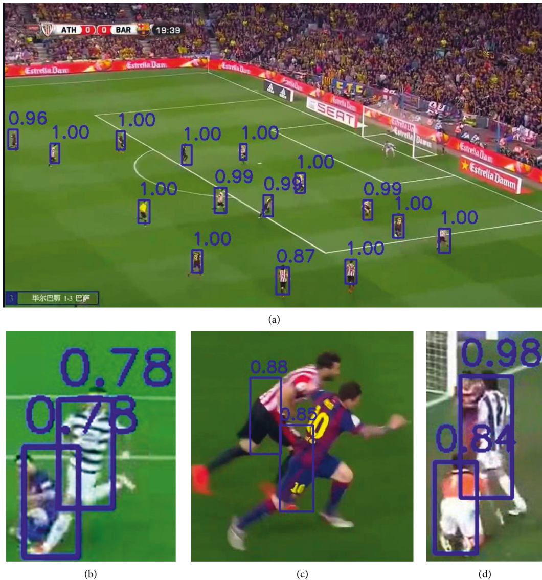
FIGURE 5: Model performance on (a) a normal football match image for player detection, and on difficult player detection tasks where players are nearby and (b) one player fell on the ground. (c) Plays' legs are overlapped. (d) One player is on his knees.
