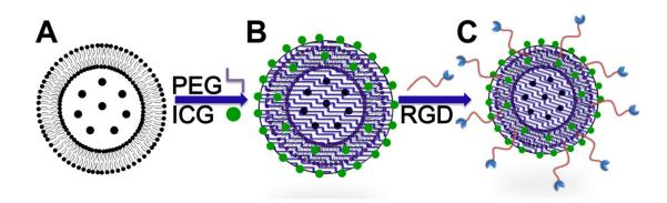
**Figure 7: Schematic diagram for the synthesis of SPIO**@Liposome-ICG-RGD. A. SPIO nanoparticles was coated with liposome (SPIO@Liposome). B. ICG molecules were loaded into the lipid layer of magnetic liposomes (SPIO@Liposome-ICG). C. RGDs were conjugated to obtain the SPIO@Liposome-ICG-RGD probes.
