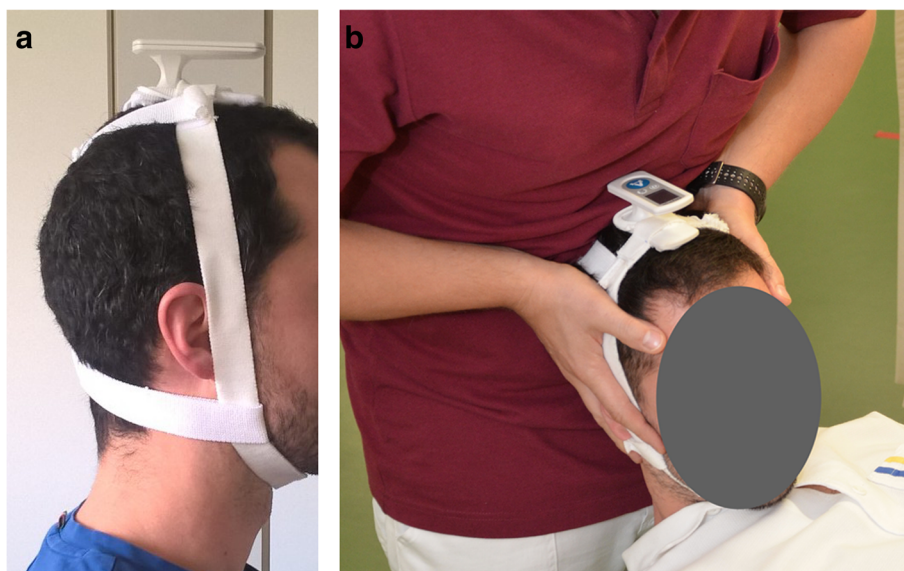
Fig. 1 a and b Reliability of the FRT measured with the easyangle. The digital goniometer was fixed via a selfmade elastic band
