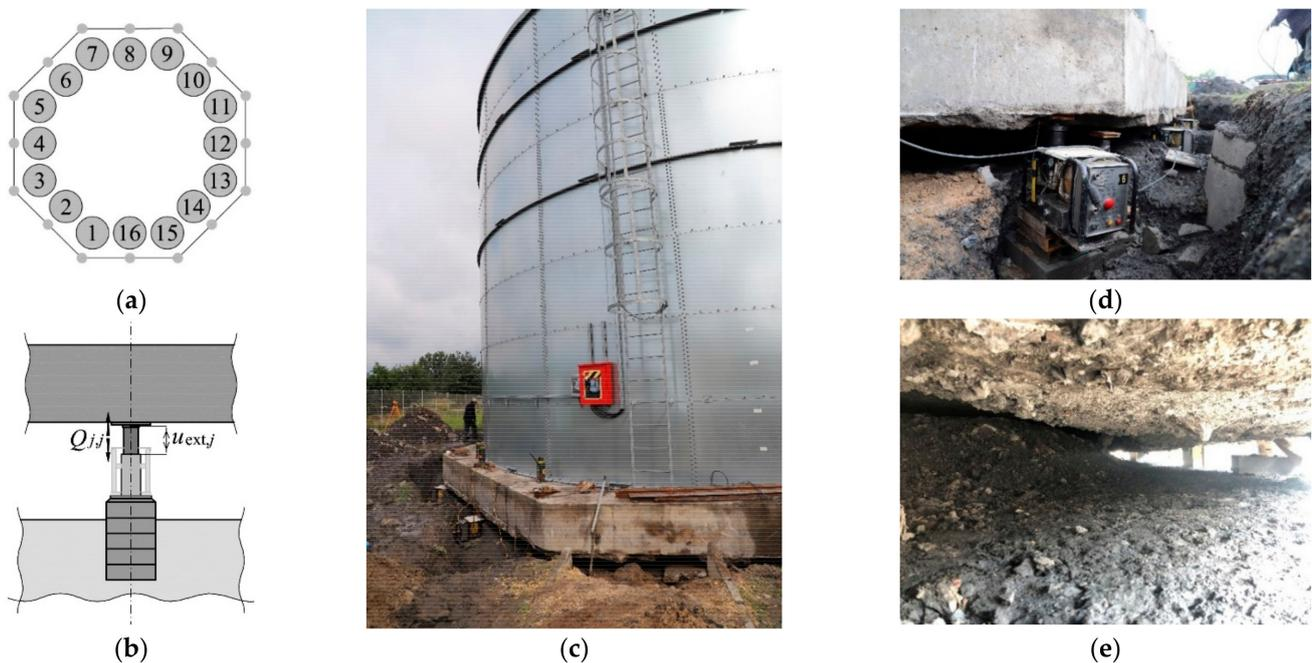
**Figure 7.** In-situ testing of stiffness  $k_{j,j}$  ( $j = 1, \dots, 16$ ), (a) positions of the installed jacks and points of measuring the values  $u_{ext,j}$  and  $Q_{j,j}$ ; (b) plan of measurements; (c) tank placed on  $n = 16$  jacks; (d) jack prepared for the tests, (e) space formed under the foundation slab after the rectification.
