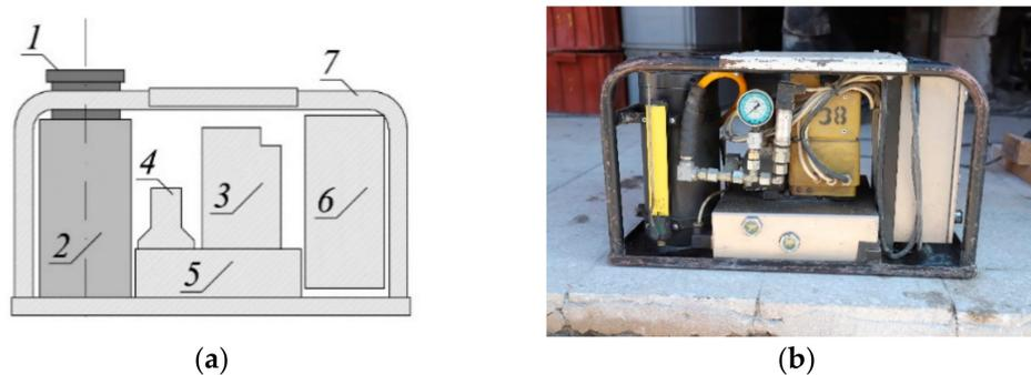
**Figure 5.** Hydraulic jack: (a) scheme; (b) view: 1—piston, 2—cylinder, 3—oil pump, 4—solenoid valves, 5—oil tank, 6—control box, 7—frame.
