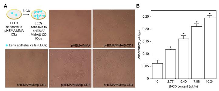
Fig 5. LEC adhesion test. (A) Inverted phase contrast microscopy of LECs that had adhered to wet samples. (B) The absorbency of LECs that had adhered to samples (shown at 630.0 nm) as a function of β-CD content (★ P<0.05 vs control). All microscopy images are at the same magnification (40 ×).
