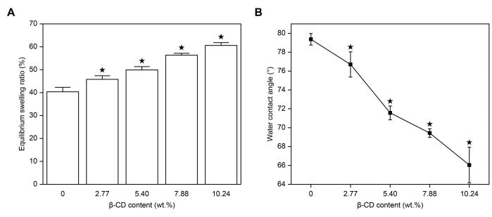
Fig 4. ESR (A) and water CAs (B) of pHEMA/MMA/β-CD hydrogels (★ P<0.05 vs control).
