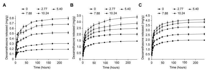
Fig 6. Total amount of dexamethasone released from pHEMA/MMA/β-CD hydrogels pre-soaked in dexamethasone solution (mg/g of dried hydrogels). The immersion conditions were (A) 0.04 mg mL<sup>-1</sup> at 25°C, (B) 0.08 mg mL<sup>-1</sup> at 25°C and (C) 0.08 mg mL<sup>-1</sup> at 37°C.
