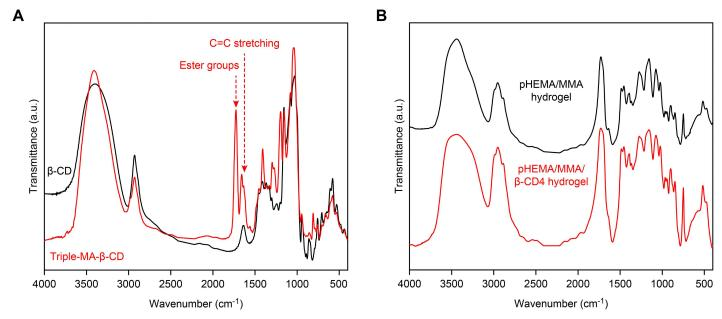
Fig 1. FT-IR spectra. (A) β-CD and Triple-MA-β-CD; (B) dried hydrogels: pHEMA/MMA hydrogel and pHEMA/MMA/β-CD3 hydrogel.
