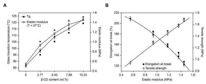
Fig 2. Thermo-mechanical properties. (A)  $T_g$  ( $\bullet$  P<0.05 vs control) and elastic modulus ( $\Box$  P<0.05 vs control) of each of the pHEMA/MMA/β-CD hydrogels as a function of β-CD content. (B) Elongation at break ( $\bullet$  P<0.05 vs control) and tensile strength ( $\Box$  P<0.05 vs control) at 37 °C relative to the elastic modulus of the pHEMA/MMA/β-CD hydrogels.
