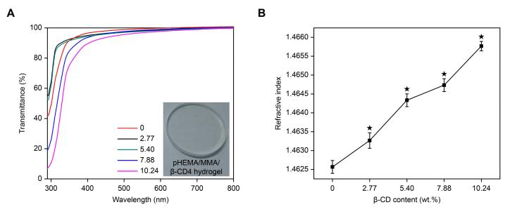
Fig 3. Optical properties. (A) Spectral transmittance of the pHEMA/MMA/β-CD hydrogels. (B) Refractive index of the pHEMA/MMA/β-CD hydrogels as a function of β-CD content ( $\bigstar$  P<0.05 vs control).
