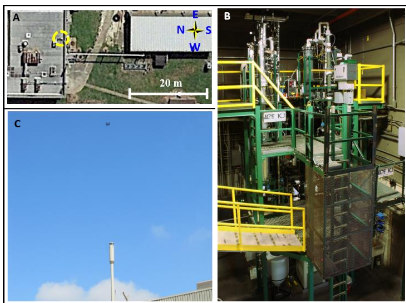
Figure 1. (A) Aerial view of the facilities employed in the University of Kentucky Center for Applied Energy (UKy-CAER). The coal flue gas generator is located to the right side and the gas flows through a polyvinyl chloride (PVC) pipe (from right to left) to the building on the left-hand side for amine treatment in the carbon capture system (CCS) before the scrubbed flue gas emissions are released out the stack at the top (yellow dashed circle). (B) Image of the amine-based CCS at UKy-CAER. (C) Perspective view of the small unmanned aerial system (sUAS) flying above the stack.
