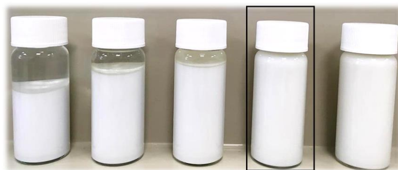
Figure 3. The HAp suspensions in PVP solutions directly after the study (from left: 0%, 5%, 10%, 15% and 20% PVP).
