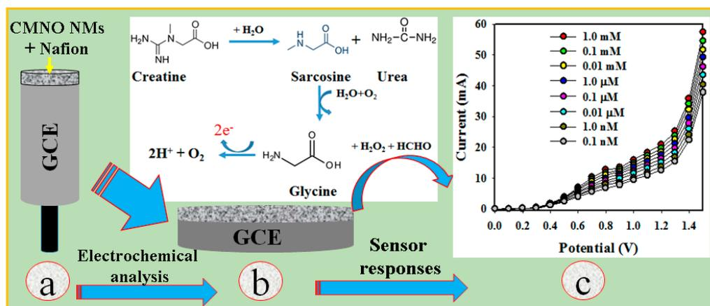
**Scheme 1.** Schematic representation of CA sensing CMNO NMs/GCE. (a) Modification of glassy carbon electrode (GCE) with CMNO NMs, (b) electrochemical oxidation of CA on CMNO NMs/GCE, and (c) responses recorded in electrometer.
