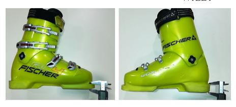
**FIGURE 1** Measuring of ski boot sole abrasion at the toe and heel piece by using a digital caliper
