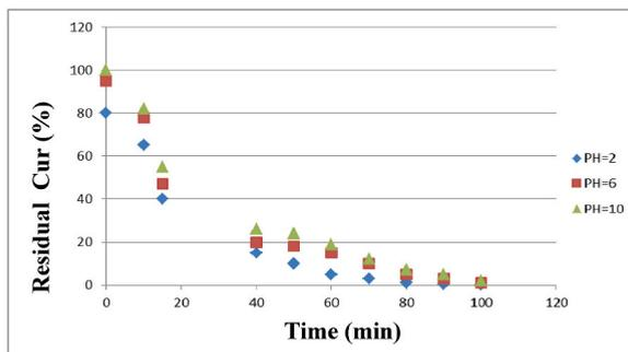
A: Kinetic degradation of curcumin (Cur) at different PH values of 0.1 M buffer solution at 35C $^{\circ}$ .
