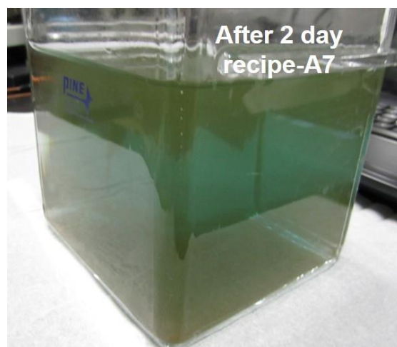
Figure S9. Photo of a degraded electrolyte bath (1 L) based on recipe-A7 after 2 days, Related to Table 2 and Figure 5
