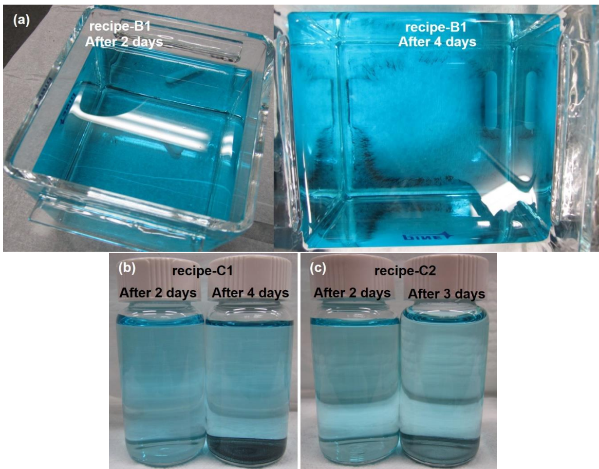
Figure S10. Photos of the electrolyte solutions based on different chemical recipes without sodium thiosulfate additive after different storage durations, showing the bath stability, Related to Table 2 and Figure 5
