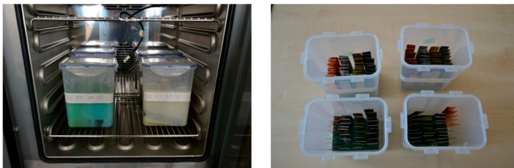
Figure 8. Metal samples prepared for corrosion testing: (left) Test beakers placed in incubator; (right) Samples in test beakers before the test.
