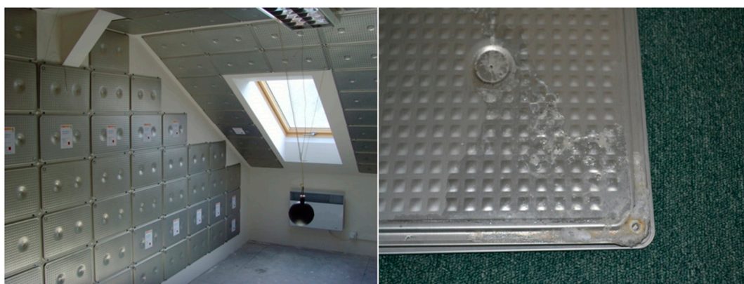
Figure 1. Application of PCM encapsulated in aluminum container: (left) Experimental installation in the test room at the Faculty of Civil Engineering, Brno University of Technology; (right) PCM leakage on the surface of aluminum container with salt hydrate PCMs placed on the wall of the test room for three years.
