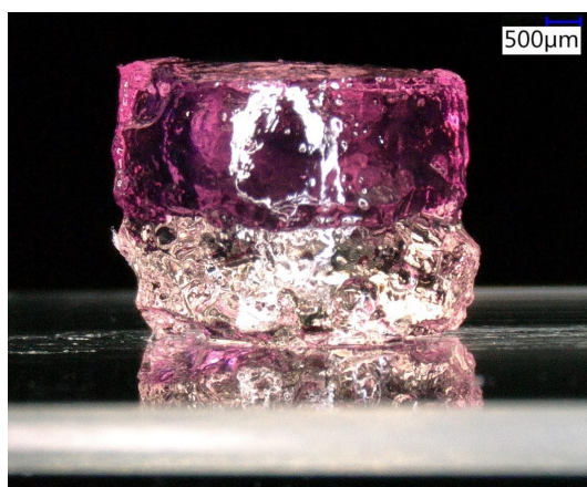
Figure 2. Concept of our stacked hydrogels cast on a standard microscope slide. Photo-polymerizable gelatin methacryloyl (GelMA) (transparent) on glass topped by a red-colored thermoset gelatin layer (red). The image was taken with a digital microscope (Keyence VHX-7000). The scale bar indicates 500 \mu\text{m} .
