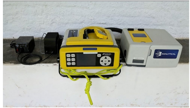
FIGURE 1 Inficon Hapsite Portable GC-MS (center) with headspace sampling systems (right), which enables analysis of solids and liquids. At left: AC power unit and voltage converter. The airprobe is shown in storage position on top of the Hapsite. Details of the fastened hoisting rope are outlined in Appendix S1
