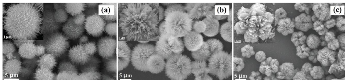
Figure 22. SEM images of the precursors of ZnO nanostructures synthesised with different dosages of urea: (a) 0.3 g, (b) 3.0 g, (c) 6.0 g. Reprinted from [654], Copyright (2014), with permission from Elsevier [OR APPLICABLE SOCIETY COPYRIGHT OWNER]. All rights reserved. In order to re-use permission must be obtained from the rightsholder.
