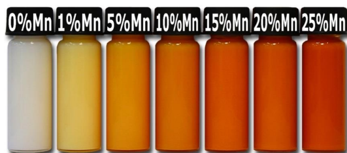
Figure 43. Visual comparison of changes in colours of suspensions of Zn_{1-x}Mn_xO NPs depending on the dopant content. Reprinted with permission from [802]. Copyright ©2016 Wojnarowicz et al. Article licensed under a CC BY 2.0, https://creativecommons.org/licenses/by/2.0/ .
