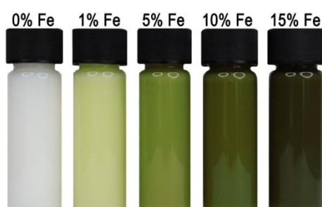
Figure 45. Visual comparison of changes in colours of suspensions of Zn_{1-x}Fe_xO NPs depending on the dopant content. Source: own test results.
