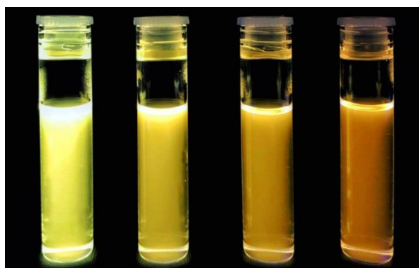
Figure 47. Photograph of oleate-stabilised ZnO NPs, dispersed in cyclohexane, under UV light ( \lambda = 365 nm) in order of increasing synthesis temperature of 125 °C (2.6 nm), 150 °C (2.7 nm), 175 °C (3.1 nm), and 200 °C (3.8 nm) (left to right). Reprinted (adapted) with permission from [795]. Copyright © 2019, American Chemical Society. All rights reserved. In order to re-use permission must be obtained from the rightsholder.
