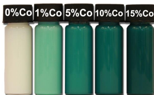
Figure 44. Visual comparison of changes in colours of suspensions of Zn_{1-x}Co_xO NPs depending on the dopant content. Reprinted with permission from [799], Copyright ©2015 Glass Ceram (Warsaw, Poland).
