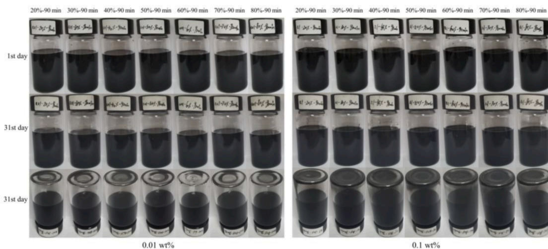
Fig. 3. Photographs of FLG nanofluids prepared at different ultrasonication powers as prepared and after a month from preparation.
