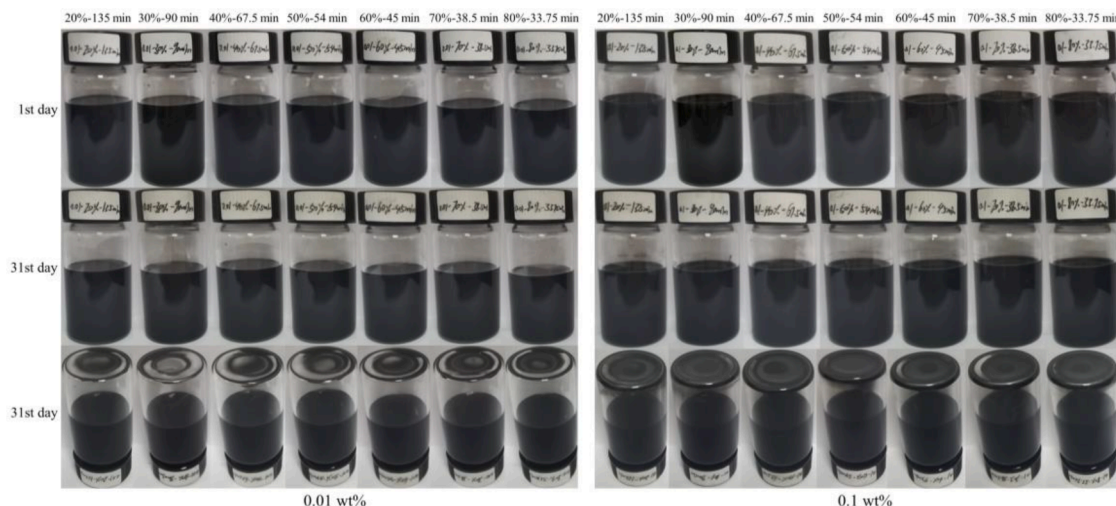
Fig. 6. Photographs of FLG nanofluids as prepared and after a month from preparation under the constant ultrasonic energy consumption condition.
