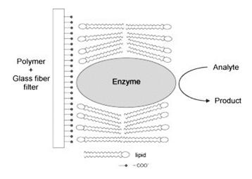
Figure 2. Schematic diagram of the lipid film-enzyme biosensor (with permission from ref. [14]).
