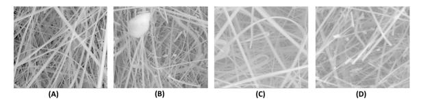
**Figure 3.** SEM images of (**A**) polymer without the lipid, (**B**) polymer with the lipid, (**C**) polymer with the lipid after the incorporation of Anti-STX, and (**D**) same as (**C**) but a drop of toxin is placed on the filter. Magnification is  $2000 \times$  (nm). (With permission from ref. [15]).
