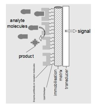
Figure 1. Schematic of a lipid membrane-based biosensor.
