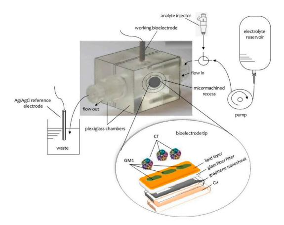
Figure 5. Schematic of the experimental set-up and the bioelectrode edge surface. (Reprinted from ref. [50]).
