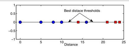
**Figure 2 Illustration of the distance threshold.** The distance threshold is chosen such that it divides the dataset into two separate groups (red and blue groups). It is clear that there is no unique best threshold. Any threshold between 10 and 14 or between 16 and 21 has only either one false negative or one false positive. However, there is no perfect threshold that separates the datasets into two pure groups.
