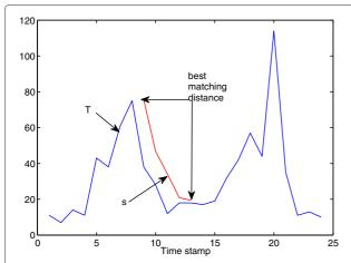
**Figure 1 Illustration of computing the distance between a subsequence s and a time series** *T***.** To compute the distance between a subsequence *s* of length 5 and a time series *T* of length 24, a window of length 5 is slid over *T* and the distance between *s* and *T* is computed as the minimum distance between *s* and every subsequence of *T* with length 5.
