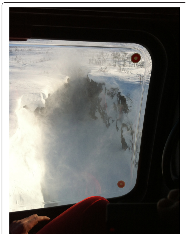
Fig. 7 Low level flight over canyon. Low level flight over canyon with manned helicopter (EC 135). Downwash causes snow to swirl up, thereby restricting visibility. Photo shot from inside the helicopter. (Photo: Håkon B. Abrahamsen)
