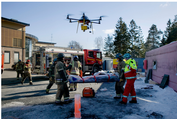
Fig. 6 Remote sensing from a simulated major incident. Remotely piloted aircraft flying over a simulated major incident. A multiprofessional rescue team (front) working on the evacuation of a trauma patient from an overturned bus (right). The transmitting antenna that caused electromagnetic interference can be seen on top of the roof in the background. (Photo: Adrian Johansen)
