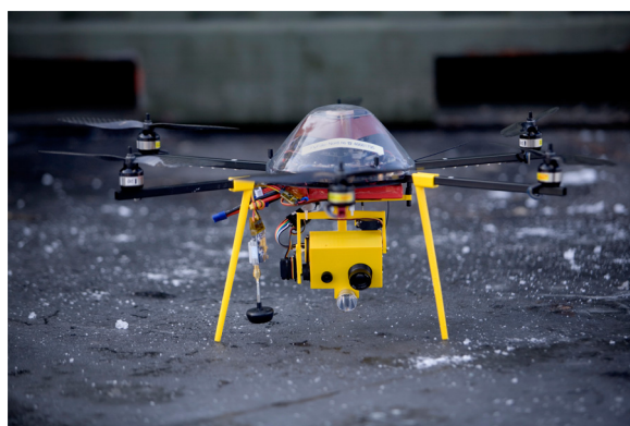
Fig. 3 Remotely Piloted Aircraft (RPA). Radio controlled multirotor unmanned aerial vehicle with searchlight and video camera. (Photo: Adrian Johansen)
