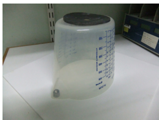
Figure 1. A plastic domestic jug converted for use as a hyponeophagia testing unit. Sweetened condensed milk can be placed in the small food well located inside the spout, which conveniently directs the attention of the mouse straight to it. The lead weight glued to the inverted base of the jug helps to stabilise it against any movement of the mouse against the walls.
