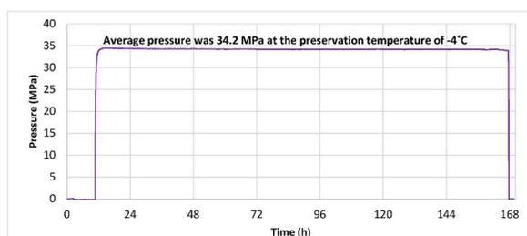
**Fig. 3.** This figure shows the pressure measurement over time (7 days) during the black grape preservation experiment in the isochoric system. During the experiment, the pressure transducer in Fig. 1A was used to measure the pressure in the isochoric chamber.
