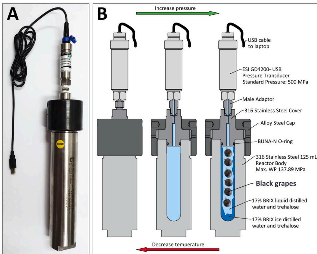
**Fig. 1.** (A) Photograph of the isochoric system, consisting of the high-pressure reactor, the pressure transducer, and the USB cable for connection to the laptop. (B) Illustration of the grape preservation process using the isochoric reactor and generalized freezing.
